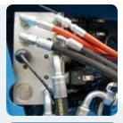
Hydraulic system steering via compact valve block
