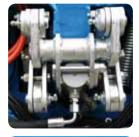
Immediate closure of both clamps in case of hauling cable break (2 sec.)
